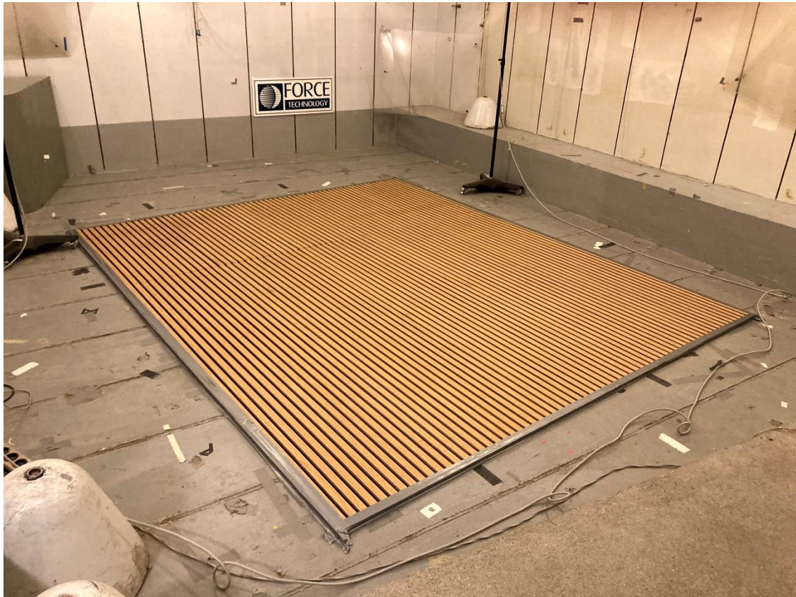
Figure 1 Acupanel FR-panels mounted in the laboratory (Type A mounting).
