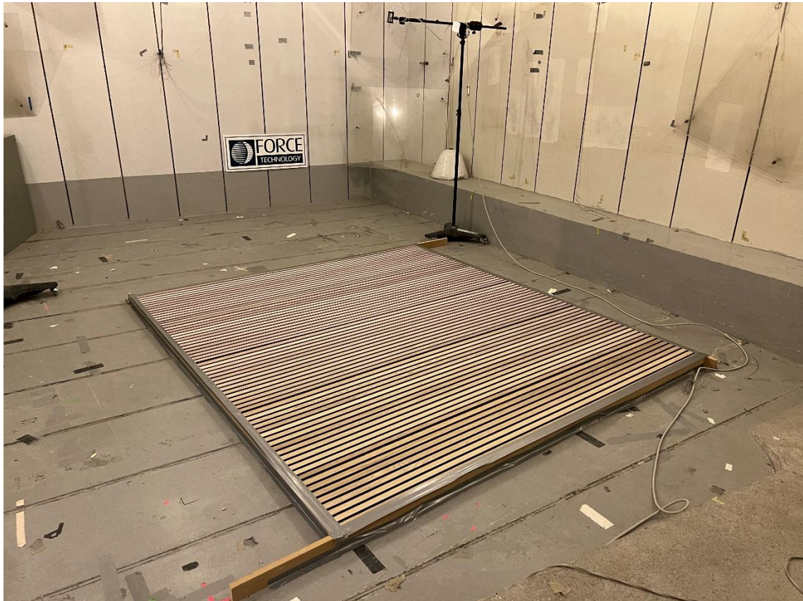
Figure 1 Acupanels Upcycled Turf Panels mounted in the laboratory (type C-45 mounting).
