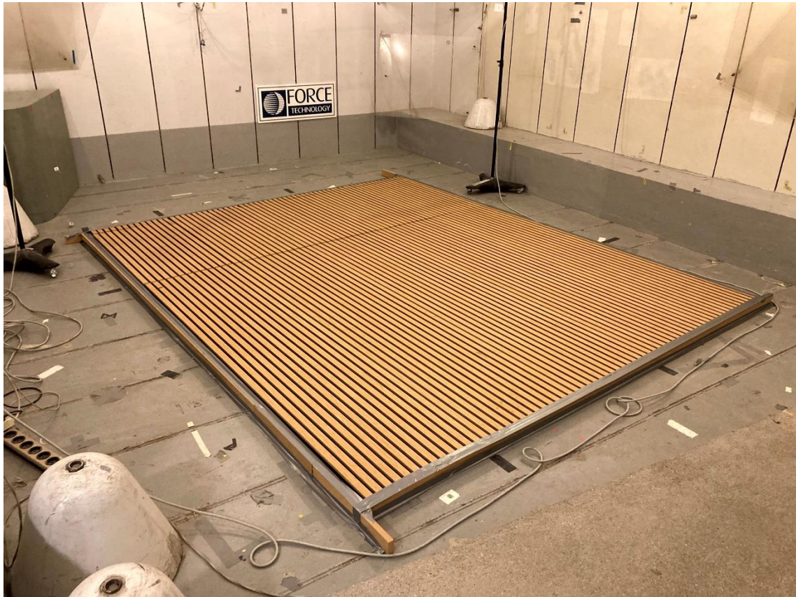
Figure 1 Acupanel FR-panels mounted in the laboratory (Type E-65 mounting).
