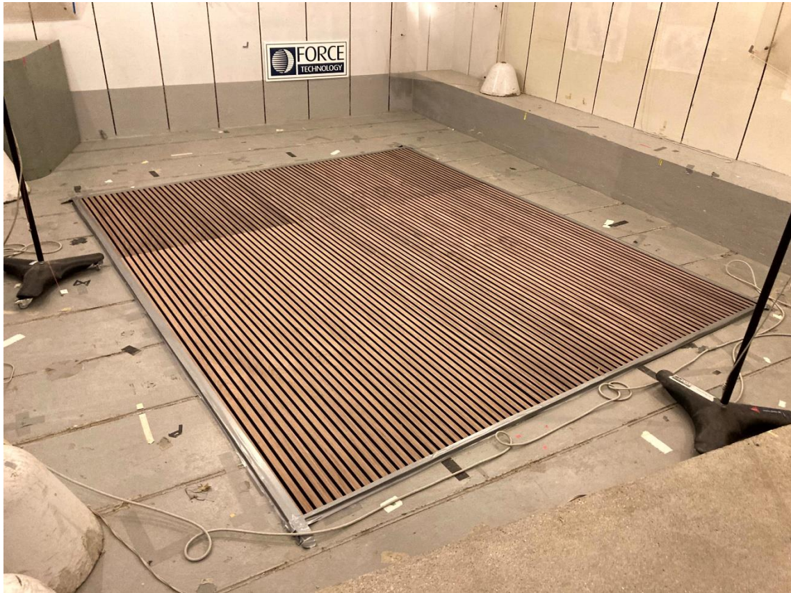
Figure 1 Acupanel Træ Panels mounted in the laboratory (Type A mounting).
